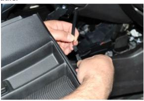
Step 20: Test system. LED light will illuminate Blue once accessories are on. Once Qi equipped device is placed on Freedom Charge LED will illuminate Green and charging begins. \*Please note on some devices syncing may take up to 15 seconds. Coil locations vary on various devices; move device on mat until LED illuminates green.
