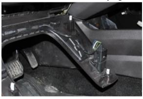
Step 18: Splice Red wire of Power Harness to the Blue (12v ignition) wire of the interior sensor plug.
