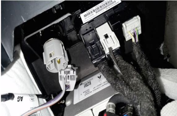
**Step 9:** On the power harness included with the Freedom Charge cut off the ringlet on the black wire (ground).
