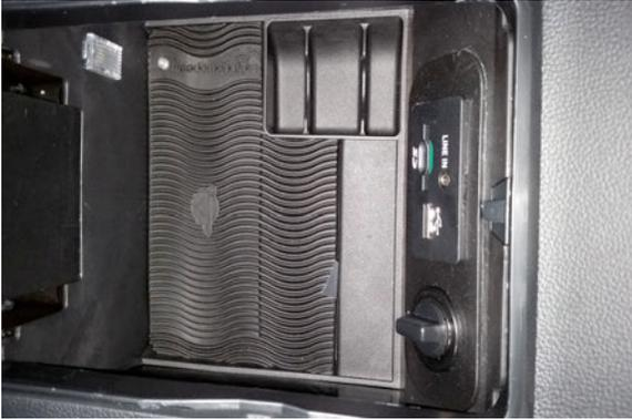
**Step 20:** Test system. LED light will illuminate blue once accessories are on. Once Qi equipped device is placed on Freedom Charge LED will illuminate Green and charging begins. \*Please note on some devices syncing may take up to 15 seconds. Coil locations vary on various devices; move device on mat until LED illuminates green.
