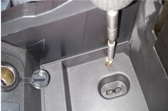
**Step 14:** Run the power harness that was connected to the power point into the 1/2 hole that was just drilled in the step 13.
