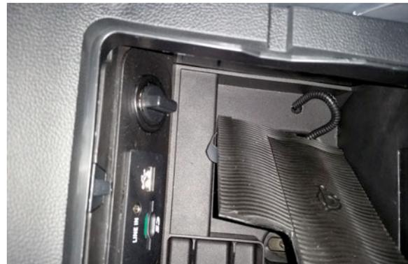
**Step 18:** Check to ensure the power harness or factory wiring is not going to be pinched lower than the console and reinstall the (2) 10mm nuts.
