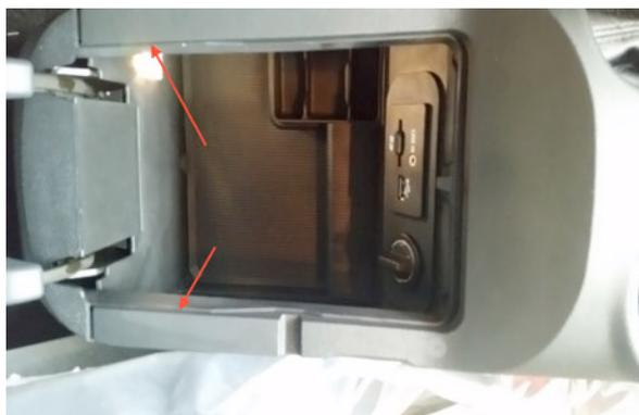
**Step 6:** Lift up from rear of console to unclip the top of console. Ensure the front of console side is pulled out slightly.
