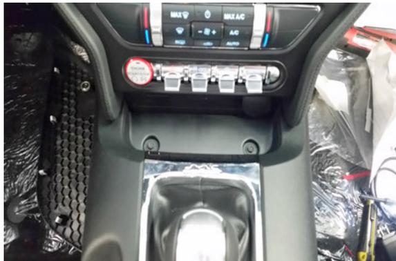
**Step 5:** Use a plastic trim removal tool to loosen the console top trim from inside the armrest.
