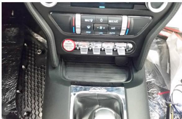
**Step 4:** Remove (2) 7 mm sockets from under rubber tray. Removal is not required but it does help with lifting the top of console.
