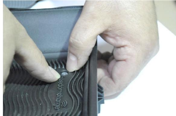
**Step 17:** Connect the Freedom Charge plug to the power harness that was run to the armrest. Pull as much excess power harness back into the underside of the console. Remember to leave a little to reinstall the (2) 10 mm nuts.
