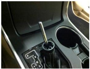
**Step 3:** Use a plastic trim removal tool and remove rear console bin.
