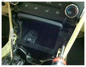
**Step 8:** Pull out console bin and disconnect USB connector.
