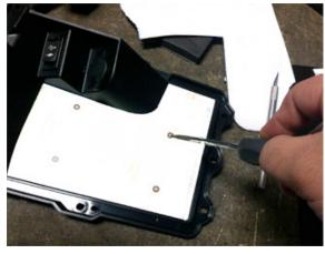
**Step 14:** Drill 1/4" hole, (4) 1/8" and (4) 3/16" holes in previous marked locations.
