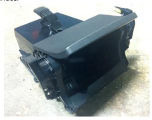
**Step 11:** Carefully flip console bin over and using a Phillips screwdriver remove (7) Phillips screws.
