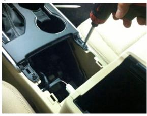
**Step 5:** Use a plastic trim removal tool to remove cup holder / shifter bezel.
