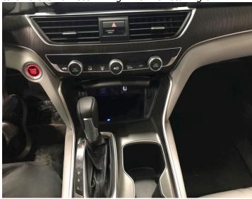
**Step 13:**Test system. LED light will illuminate blue once accessories are on. Once Qi equipped device is placed on Freedom Charge LED will illuminate green and charging begins. \*Please note on some devices syncing may take up to 15 seconds. Coil locations vary on various devices; move device on mat until LED illuminates green
