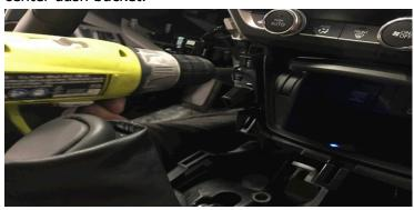
**Step 6:** After removing center dash bucket locate the bottom and use supplied template and mark 12 grid squares for removal in picture below.
