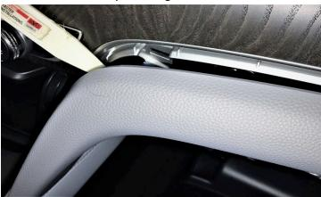
**Step 3:** Using a plastic trim removal tool remove both sides of center console.
