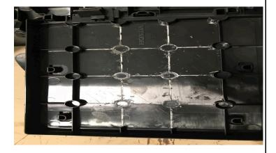
**Step 8:** Make sure plastic is sanded flat for proper Freedom Charge mounting.
