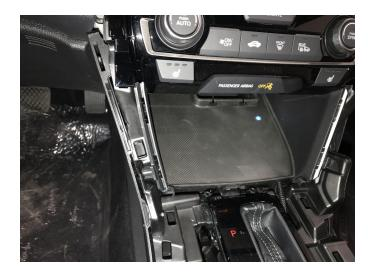
**Step 10:** Reassemble vehicle. Follow your disassembly steps in reverse order, taking care not to bind the harness wiring when reinstalling
