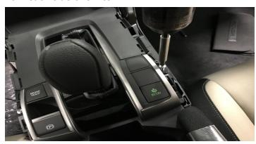
**Step 3:** Using a plastic trim tool remove trim panel around shifter.
