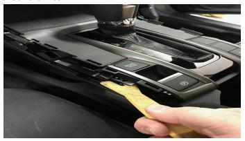
**Step 4:** Using a plastic trim tool remove center plastic cover in front of shifter.
