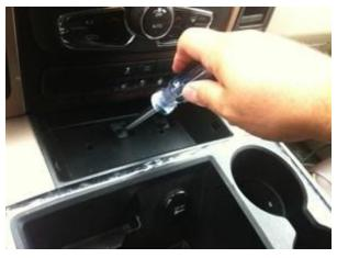
Step 3: Use a Plastic Trim Removal Tool to remove chrome surround trim. ( DO NOT REMOVE THE CHROME TRIM RING ON 2016 AND UP TRUCKS, THIS TRIM DOESN'T REMOVE.)
