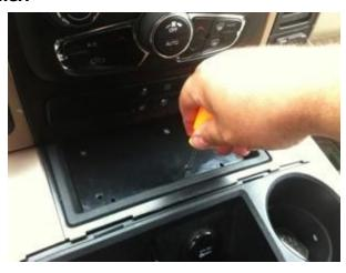
Step 14: Swing Charging Module away and Drill (2) 1/8" holes through rubber tray liner and upper console trim.
