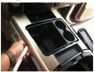
Step 5: Cut out provided template and mark location for 1/2" hole.
