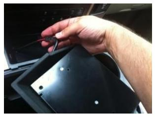
Step 12: Place Freedom Charge Module and rubber tray liner into upper console trim. Make sure to fully snap in rubber liners
