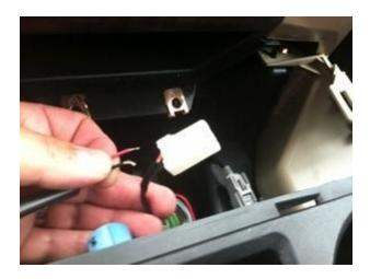
Step 9: Route black connector of Charging Module through 1/2" hole of rubber tray liner.
