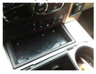
Step 13: Using a center punch/scribe tool mark the location of the (2) chamfered holes through Charging Module onto rubber tray liner.
