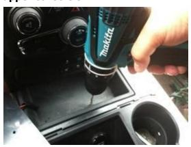
Step 15: Insert the (2) 1" Flat Head T-10 Torx Screws through Charging Module and rubber tray liner into upper console tray.
