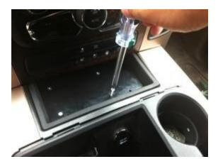
**Step 16: Install Non-Slip Freedom Charge Mat to Wireless Charging Module.** Place the 4 locator pins in corresponding holes.
