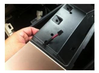
**Step 11: Connect Power Harness to Charging Module.**
