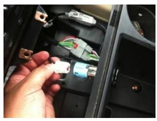
Step 8: Splice Red wire of Power Harness to the Red/Yellow (12v ignition) wire of the power point plug and Splice Black wire of Power Harness to the Black (ground) wire of the power point plug
