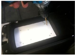
Step 3: Use 82° Chamfer bit to chamfer the (4) 3/16" holes. An X-acto knife can be used by laying it down on its side and removing material around the hole.
