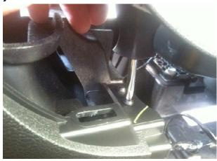
**Step 11: Using Trim Removal Tool loosen side console trim.**
