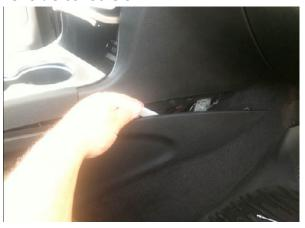
**Step 13: Using 7mm Nut Driver remove 7mm nut,**
