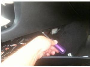
Step 14: With trim loosened reach behind keyed power point and disconnect at connector.
