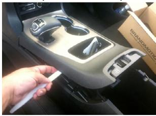
Step 10: Using Phillips Screw Driver remove (2) screws attached to side covers.
