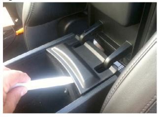
Step 7: Using Phillips Screw Driver remove (2) screws attached to side covers.
