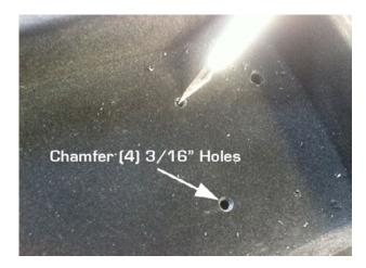
Step 4: Lift up armrest tray and place FreedomCharge module with LED poking through 5/16" hole. Then align the (4) 3/16" holes with mounting holes on module.
