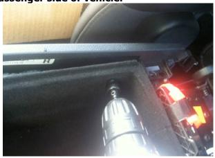
Step 15: Run harness through 1/2" hole into armrest bin.
