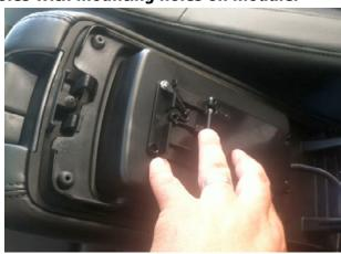
Step 5: Insert the (4) 1/2" Flat Head T-10 Torx Screws through top of tray and into FreedomCharge module.
