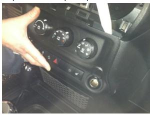
**Step 17:** Splice Red wire of Power Harness to the Blue/Red (12v ignition) wire of the keyed accessory power point plug and Splice Black wire of Power Harness to the Black (ground) wire of the power point plug.
