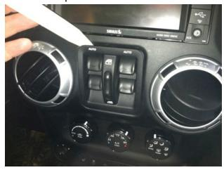
**Step 11:** Disconnect harness from window switches.
