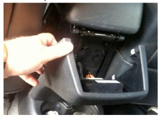
**Step 7:** Drill 1/2'' hole through lower armrest bin side panel  $1 \frac{1}{2}''$  below top lip on passenger side of vehicle.
