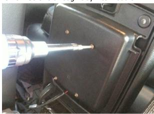
**Step 5:** Using Trim Removal Tool remove hinge cover.
