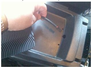
**Step 4:** Align the (4) 3/16" holes with mounting holes on module and insert the (4) 3/8" Pan Head T-15 Torx Screws through tray into module.
