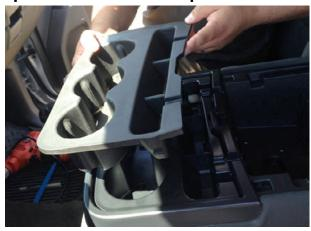
**Step 12: Using Phillips Screw Driver remove** (2) screws in cup holder and remove.
