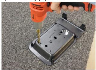
Step 6: Route connector of Charging Module through 1/2" hole and place module in tray.
