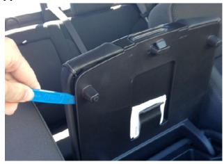
Step 2: Using a Phillips Screw Driver remove (4) screws to remove upper armrest tray.
