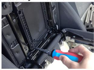
**Step 11: Remove rubber cup holder liner.**
