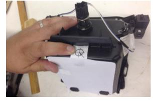
Step 6: Drill 1/2" hole in marked location.
