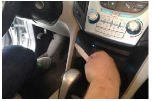
**Step 2: Use 7mm Nut Driver to remove the** (4) 7mm nuts.
