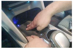
**Step 14: Reassemble vehicle**. Follow your disassembly steps in reverse order, taking care not to bind the harness wiring when reinstalling trim.
