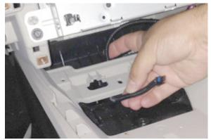
Step 9: Route Plug of Charging Module through 1/2" hole and place module in bin.
