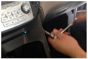
**Step 3: Slide Plastic Trim Removal Tool under** floor of bin to help slide out
