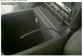
Step 16: Drill ½ inch hole in underside armrest lid as shown.
