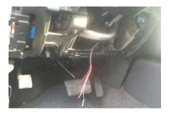
Step 21: Splice Red wire of Power Harness to the Brown (12v accessory) wire of the BCM located under the driver dash left of the steering column, Light Green Plug pin 21. RECOMMENDED: Solder wires and cover with Heat Shrink Tubing.
