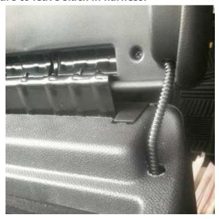
Step 19: Drill ½ inch hole in underside armrest lid as shown.
