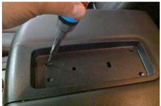
Step 2: Using Phillips screwdriver remove upper armrest underside lid.
