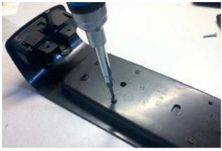
Step 9: Drill the (1) 1/2" hole in rear driver side of lid as shown.
