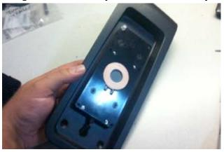
Step 8: Align the (4) 3/16" holes with mounting holes on module and insert the (4) 3/8" Pan Head T-20 Torx Screws through tray into module.
