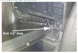
**Step 20: Route Power Harness forward under driver side dash and remove cover.**
