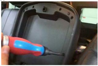
Step 3: Using a Phillips Screw Driver remove screws to remove upper armrest tray.
