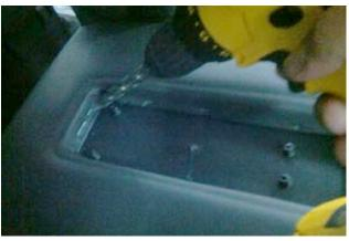
Step 10: Route connector of charging module through 1/2" hole and place top tray back to original location.
