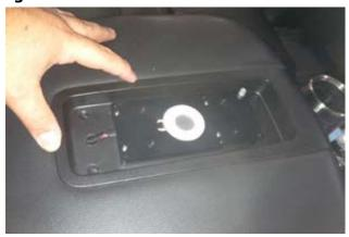
Step 11: Using a Phillips Screw Driver reassemble top tray.
