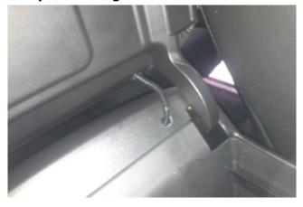
Step 14: Route Power tuck under driver side of console towards vehicle BCM located under driver side dash.
