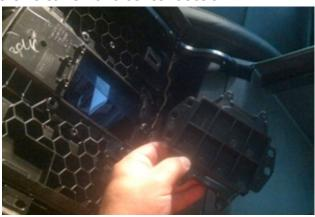
**Step 4: Cut out Trim Template and remove** material indicated area with roto tool or file.
