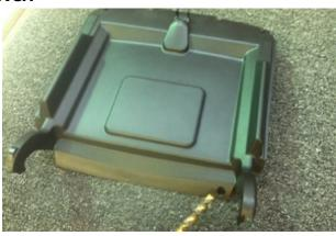
Step 10: Remove rear cup holders and unscrew torx screws to loosen rear console cover.
