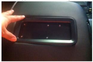
**Step 7: Using a Torx Screw Driver reattach screws to upper armrest trim ring.**
