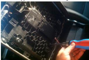
Step 8: Install Non-Slip Freedom Charge Mat to Wireless Charging Module. Place the 4 locator pins in corresponding holes.
