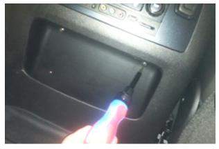
Step 11: Drill ½" hole on driver side of rear console cover.
