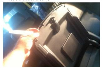
Step 2: Using a Torx Screw Driver remove screws to remove upper armrest trim ring.
