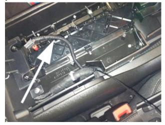
Step 13: Reattach upper armrest tray using Phillips Screw Driver. Make sure Power Harness is through the 1/2'' hole.
