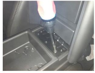
**Step 4: Using a Phillips Screw Driver remove** (2) screws under armrest hinge.
