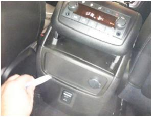
**Step 8: Using a Trim Removal Tool remove rear console trim panel.**
