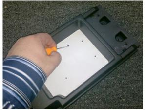
Step 7: Using a Trim Removal Tool loosen upper console trim panel.
