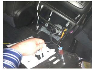
Step 10: Splice Red wire of Power Harness to the Pink (12v switched ignition) wire of the keyed USB connector and Splice Black wire of Power Harness to the Black w/ White Stripe (ground) wire of the USB connector.
