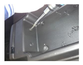
Step 3: Using a Phillips Screw Driver remove (5) screws at armrest hinge.
