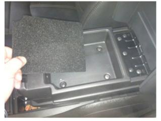
Step 2: Using a Phillips Screw Driver remove (6) screws in armrest tray.
