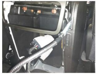
Step 12: Pull Power Harness though opening in sliding armrest tray lower and secure with zip tie.
