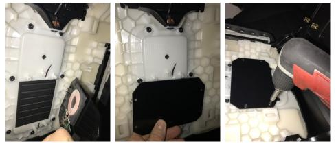
5. Connect power harness to new replacement charging module and snap panel back in place.
