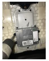
4. Orient the replacement charging coil so that it is facing the matt on the top edge. Use saved screws to secure replacement module to armrest. (Add optional spacers to offset coil) Check from the top side of the armrest to see if the new plate needs to be spaced lower ie... coil is pushing up into rubber mat.
