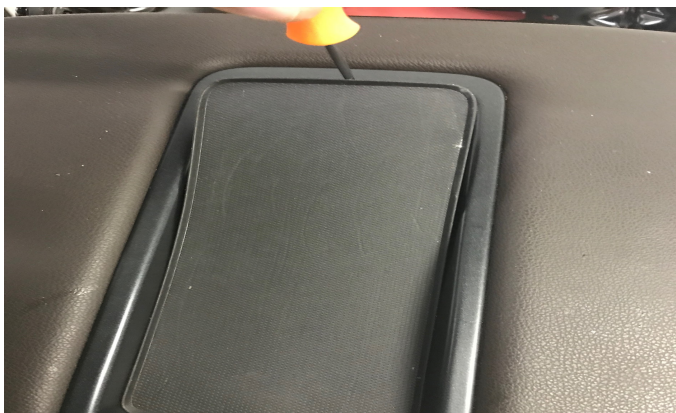
Step 3: Using a Torx Screwdriver remove screws to remove upper armrest trim ring.
