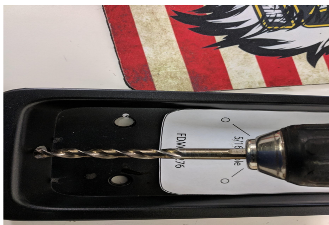
Step 6: Drill 3/8 inch hole for Power Connector at rear center of trim ring.
