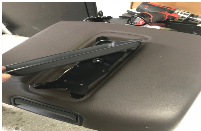
Step 5: Using template drill the four marked holes. 1/8 inch front holes 5/16 inch rear holes.
