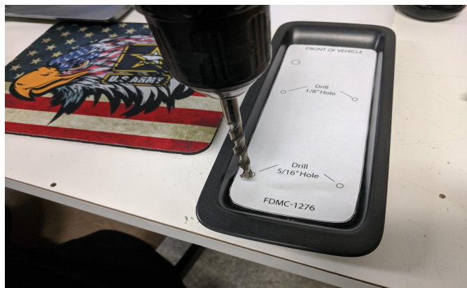
Step 5: Using template drill the four marked holes. 1/8 inch front holes 5/16 inch rear holes.
