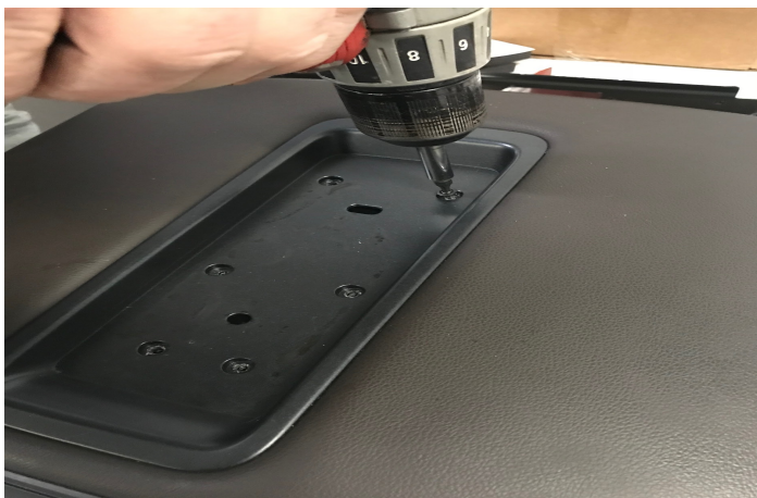
Step 4: Remove Plastic insert.
