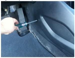
**Step 2: Remove the rubber liner from bin forward of shifter.**
