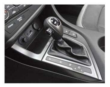
3. Start by removing the leather trim around shifter. Pull up with your fingers on the trim around the other edge of the leather.
