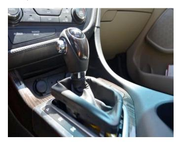
5. To remove the shifter knob, grab shifter knob, pull up and "wiggle" knob to release.
