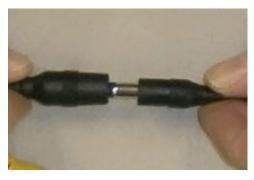
**Step 11:** Splice the red wire from the Power Harness to a 12v+ Ignition power wire in your vehicle. (Recommended: T-taps or Solder.)
