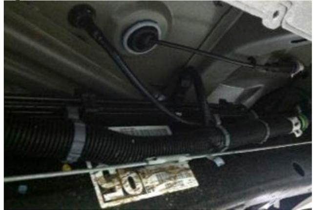
25. Connect supplied Chassis Harness to Tailgate Handle Camera harness. Use supplied glued heat shrink tube over RCA and Power connector to create seal between chassis and camera harness. (Figure 13)
