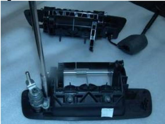
10. Route Tailgate Handle Camera connector down through Tailgate Handle opening then out through the hole at bottom of Tailgate.
