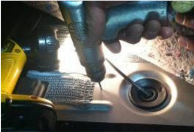
**21. Recommended:** Apply a corrosion inhibitor to the Chassis Harness pass through hole. (Figure 8)
