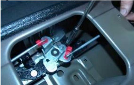
9. Remove lock cylinder from original Tailgate Handle. Remove Tailgate Lock Cylinder Retaining Clip and then Tailgate Lock Cylinder and reinstall into supplied Tailgate Handle Camera. (Figure 4)
