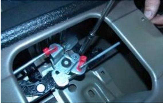
8. Remove Tailgate Handle using a Socket. (Figure 3)
