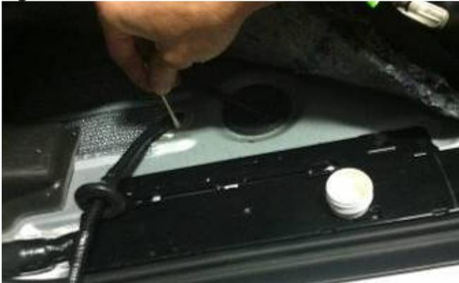
**22.** Insert RCA connector end of supplied Chassis Harness through cab floor into cab. (**Recommended:** Silicon or Grommet to seal off hole.)
