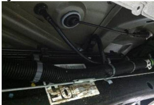
25. Connect supplied Chassis Harness to Tailgate Handle Camera harness. Use supplied glued heat shrink tube over RCA and Power connector to create seal between chassis and camera harness. (Figure 13)
