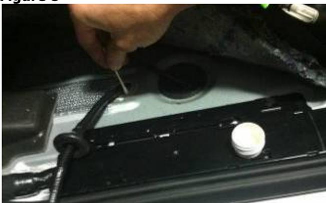
**22.** Insert RCA connector end of supplied Chassis Harness through cab floor into cab. (**Recommended:** Silicon or Grommet to seal off hole.)
