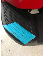
3. Remove housing base and drill three screw holes with 1/8th inch drill bit. Be sure to drill through the layer of metal beneath the plastic bumper. Using the template that was traced on the tape, cut out the hole for the connector.
