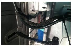
Step 12: Use a T20 Torx bit to remove subwoofer box.
