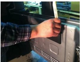
**Step 8:** Pull harness through the rear gate openings.
