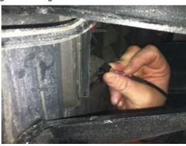
**Step 7:** Using a plastic trim removal tool, remove interior panels on inside of rear gate.
