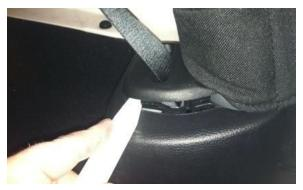
**Step 14:** Using a plastic trim removal tool, remove rear access panel to expose 10mm bolt, and remove bolt.
