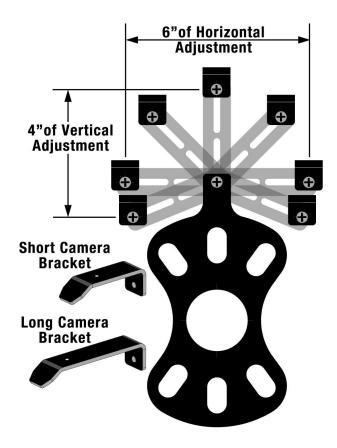
**Note:** Short Bracket has been designed for Factory offset wheels. Use the Long Bracket for wheels with larger offsets.
