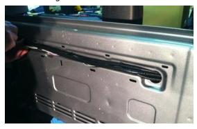
**Step 11:** Use supplied Wire Ties to secure Chassis Harness to fabric factory wire cover. CAUTION: Leave enough slack to allow gate to open fully.
