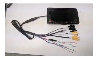
**Front & Rear Camera wiring:** Both Cameras needs 12-volt accessory power and Chassis ground from a clean non-painted surface. Also needs the composite video output cable ran to Video inputs on monitor. (1-4). Can be hooked up to desired orientation on video screen. All outside connections please use supplied heat shrink as to not VOID WARRANTY.
