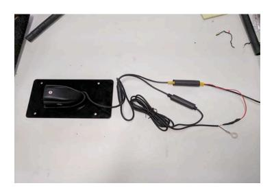
**Front & Rear Camera wiring:** Both Cameras needs 12-volt accessory power and Chassis ground from a clean non-painted surface. Also needs the composite video output cable ran to Video inputs on monitor. (1-4). Can be hooked up to desired orientation on video screen. All outside connections please use supplied heat shrink as to not VOID WARRANTY.
