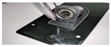
Step 4: Reassemble side view Camera. Follow your disassembly steps in reverse order
